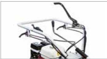
Steering with independently controlled releases and brakes.
