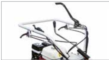
Steering with independently controlled releases and brakes.
