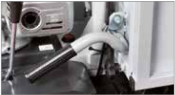
Manual dump with automatic locking system.
