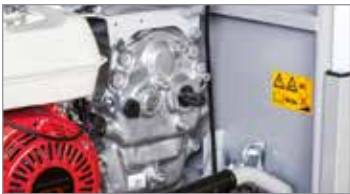
Independent PTO at 2100 rpm.
