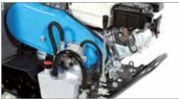
Lever-operated hydraulic tipping control valve.
